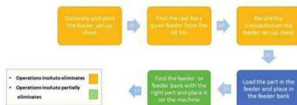
Figure 2. Typical process chart for loading feeders on the SMT machine.
